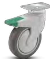
Our Directional Lock casters are designed to lock the swivel but not the wheel allowing you to steer your equipment. The directional lock feature is designed to break free under heavier load when the unit is traversing a corner only to lock back into position when the unit resumes a straight course.
