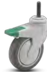
Our Directional Lock casters are designed to lock the swivel but not the wheel allowing you to steer your equipment. The directional lock feature is designed to break free under heavier load when the unit is traversing a corner only to lock back into position when the unit resumes a straight course.
