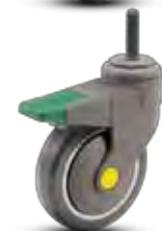
Our Directional Lock casters are designed to lock the swivel but not the wheel allowing you to steer your equipment. The directional lock feature is designed to break free under heavier load when the unit is traversing a corner only to lock back into position when the unit resumes a straight course.
